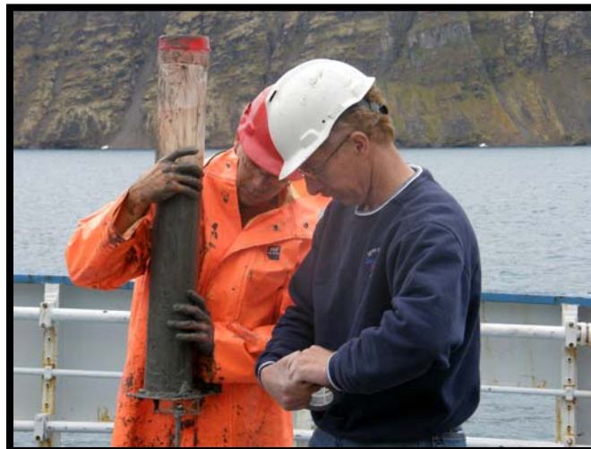
Fig. 11: Co-chief scientist Paul Loubere with NIU crew member Mathieu Richaud retrieving fjord sediments in a multicore
